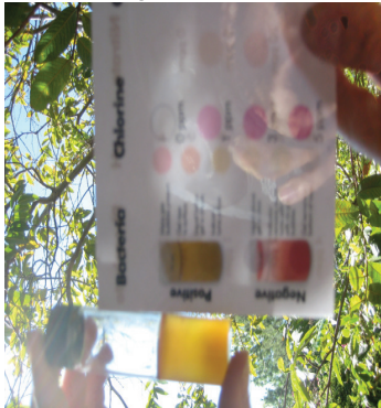
Fig. 3. PURA water test verifying bacterial contamination
